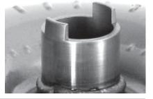
49 Size 13" Daikin Hub Geared Hub Pilot .982" OD x 1.10" L Mounting 6 Threaded Holes Stator Splines 18 Turbine Splines 19
