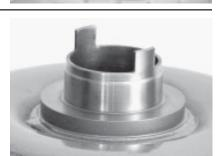
39 Size 11" Sachs Hub Slotted Hub Pilot 1.181" & 1.148" OD Mounting 4 Mounting Pads Stator Splines 38 Turbine Splines 27
