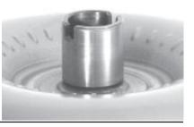
69 Size 11" Komatsu Hub 2 Flats on Hub Pilot Removable type Mounting 8 Threaded Holes Stator Splines 30 Turbine Splines 14
